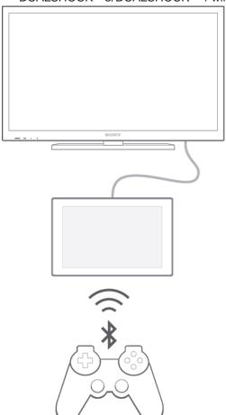
To set up a connection between a DUALSHOCK™ wireless controller and your device, a USB Host adapter is required.
